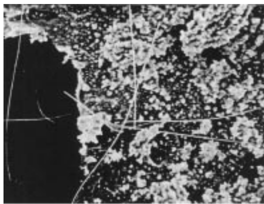
Figure 3. Scanning electron micrograph (SEM) images of a P3MeT deposit exposed to white light (1300 lx, 7 days) in a moist N 2 atmosphere. The deposit (bright region composed of a film and irregular-shaped conglomerates) was peeled off the ETO layer and then mounted on a carbon adhesive tape (dark background). The NH 4 + ClO 4 - needles with high aspect ratios are observed, some of which are curved by the electron-beam irradiation. Scale bar: 100 μm.
